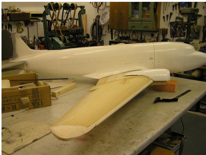
A first "coming together" some months back when we were trying to assess all up weight and C of G position. The plug on nose section is very visible
