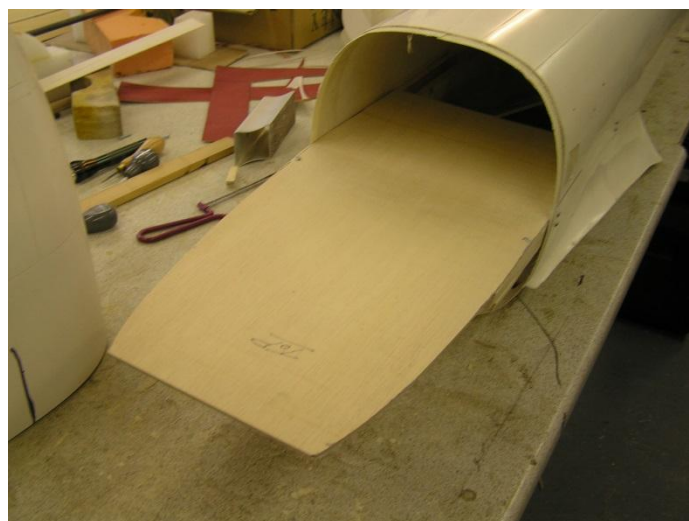
The "plug & socket" fuselage join with cantilevered battery tray.
