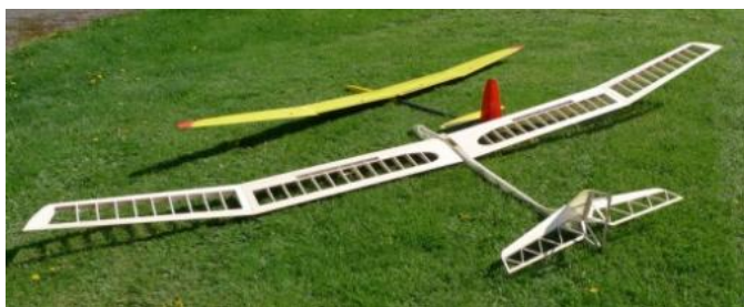
The model in frame is a Sagitta XC (Cross Country). It is 14.5 span and is a superb flier. It only has rudder, elevator and spoilers as the primary controls but doesn't lack maneuverability.
